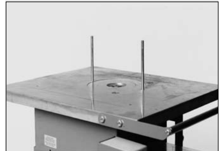
Screw both stud bolts into the tapped bore holes of the table.
